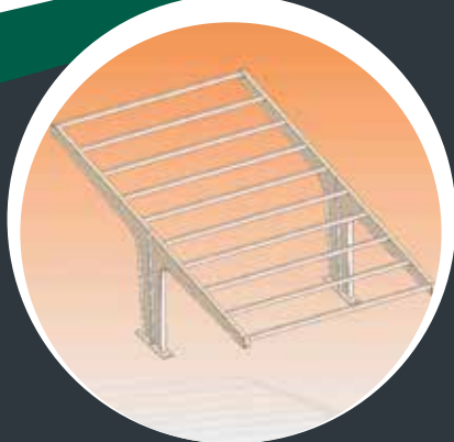
Carport for 4 parking lots without footpath is suitable for installation of 30 PV modules
